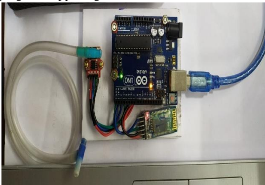
Figure 7: Hardware View of Smart spirometer using air pressure sensor
