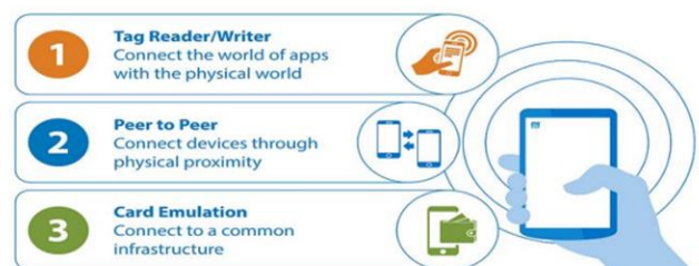
Figure 1: Modes of Operation (Sources: NFC-Forum)
